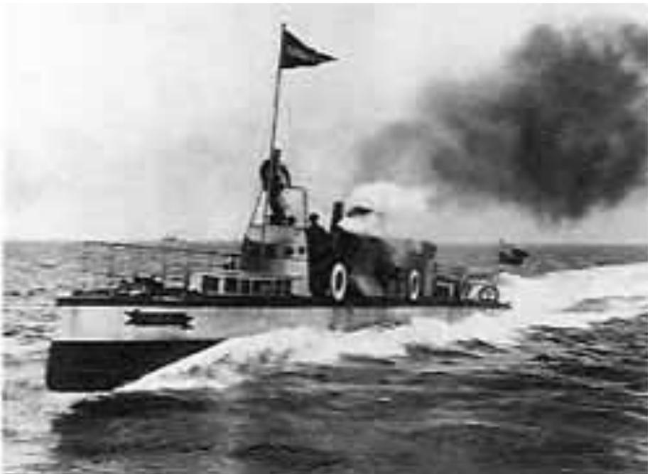
**CA Parsons' Turbinia, the first boat to be powered by a steam turbine.**
